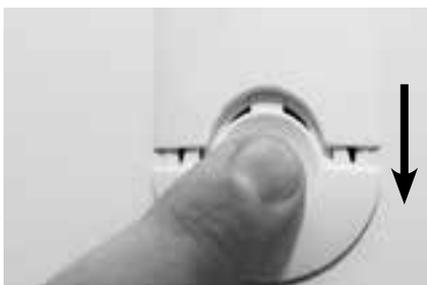
Open the inspection door by turning the two lock bolts with a screw driver for slotted screw heads. The door can then be carefully lifted off when the lock bolts have been opened.
