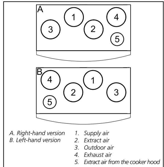
Install the ducts according to the ventilation drawings. Do not mount ducts directly against structural elements to avoid the propagation of sound.
