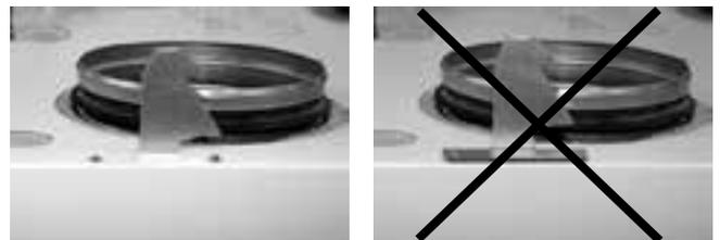
The points of the hooks face the rear part of the ventilation unit and they are to be slipped into the unit's notches before you secure them with rivets.
