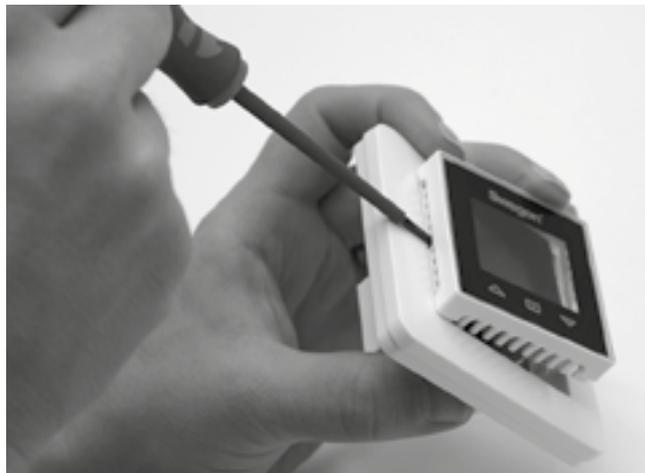
If several control panels are connected in chain, the middle panel's bus termination is moved to the "Open" position. The jumpers do not need to be adjusted if only one control panel is used.
