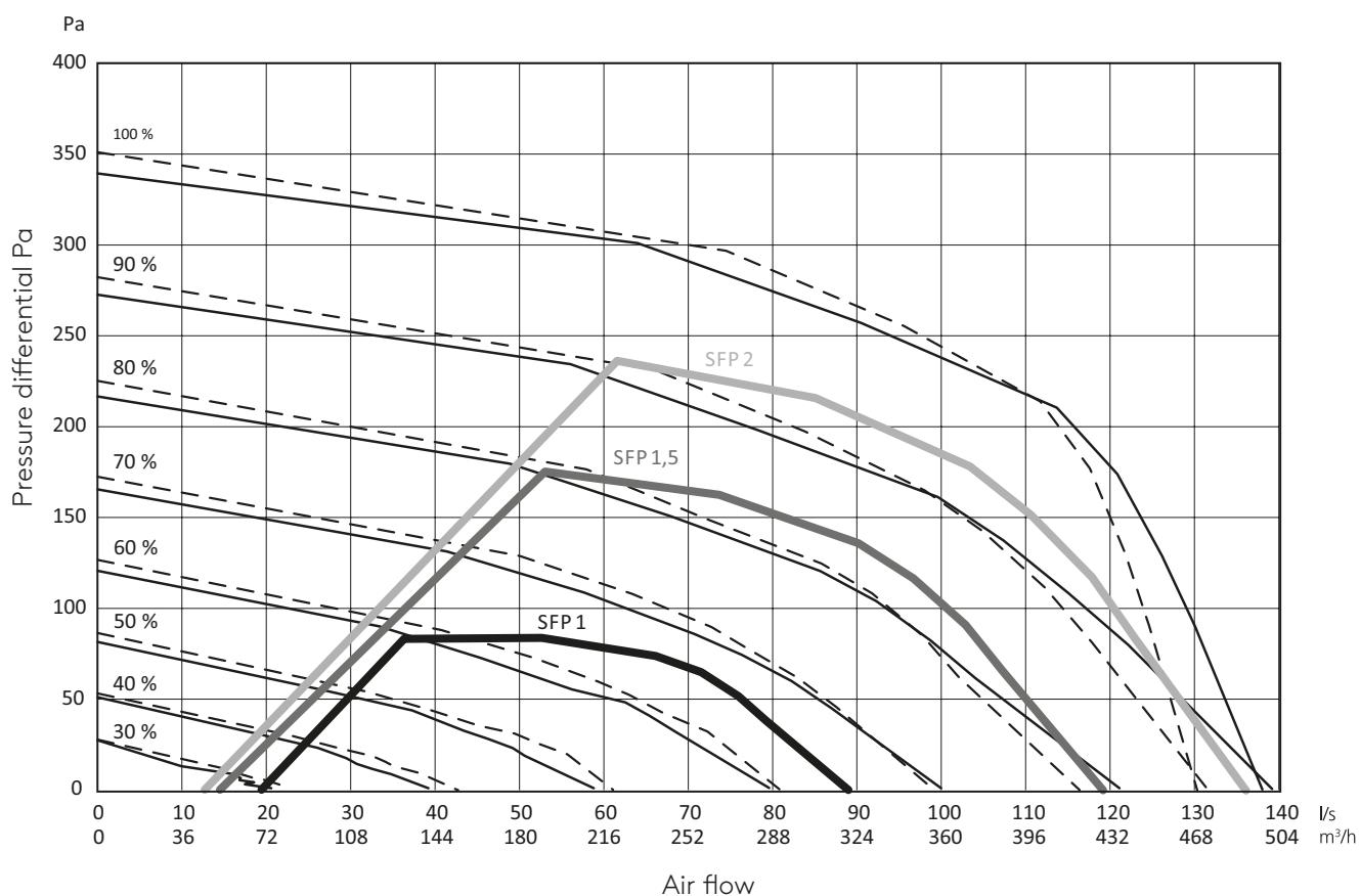
Note! If the humidity production in the apartment is high, the boost margin must be at least 30%.
