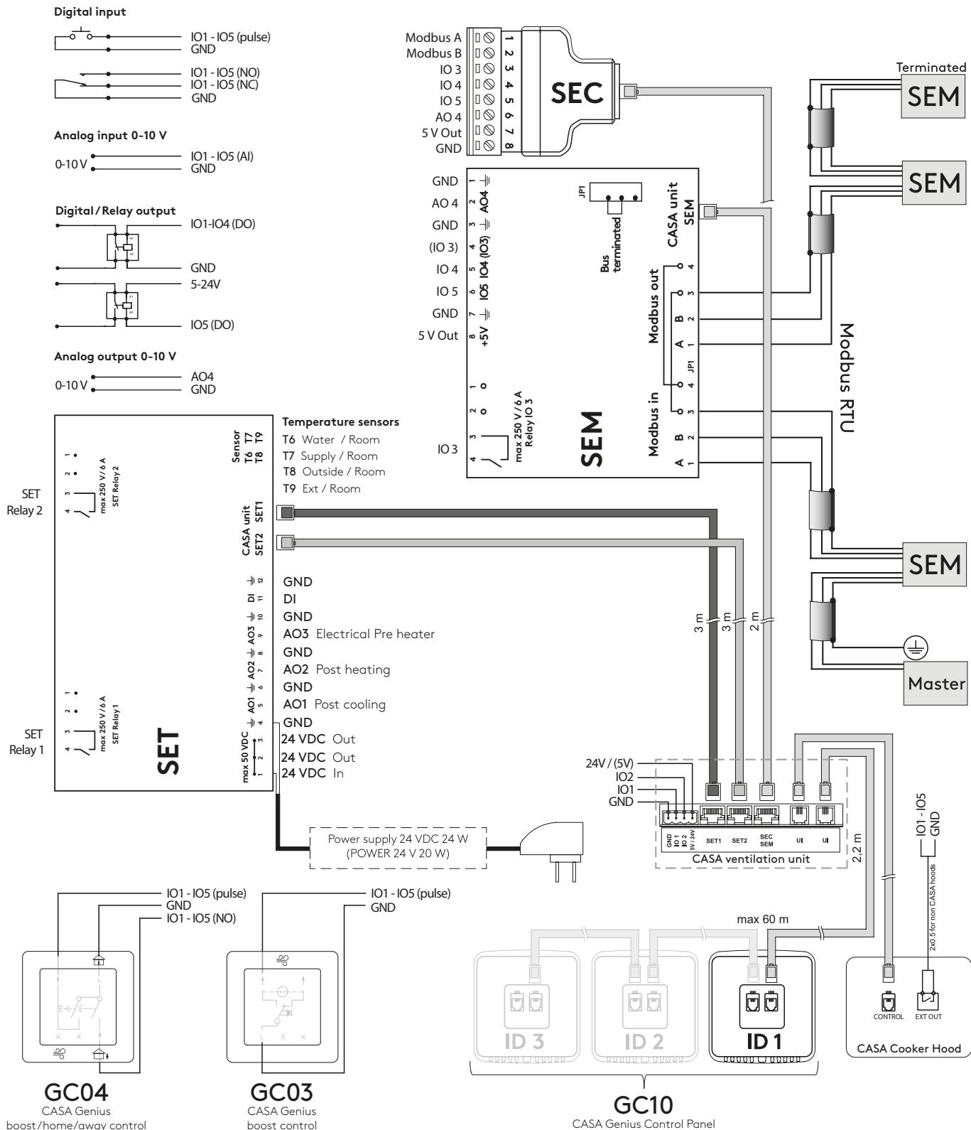
**SEC** IO extension cable with Modbus RTU
