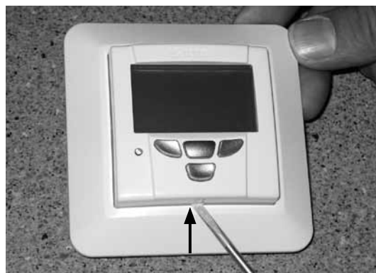
Removal of the panel from the ILTO Premium control unit.
